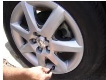
2. Position the tyre with the valve stem downwards (at 5 o'clock or 7 o'clock) and remove valve core to deflate the tyre.
