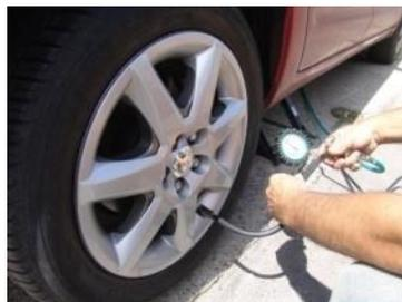
9. Inflate the tire to proper pressure (the air compressor will be equipped with clean and dry air filter to prevent water or dust entry into the tire).
