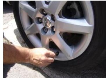
8. Reinstall the valve core.
