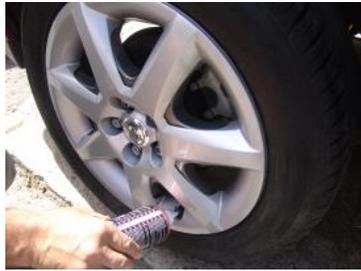
7. Place the top of the cap inside the valve and squeeze the bottle to insert the required amount of FK.
