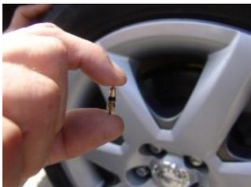
3. Valve core is completely removed before FKR installation.
