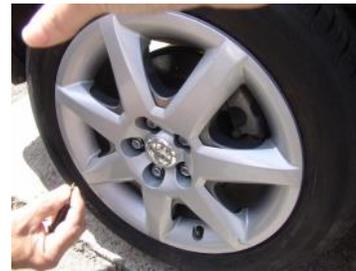
4. Deflate the tyre (to atmospheric pressure) , until you don't hear the air coming out from the tyre.
